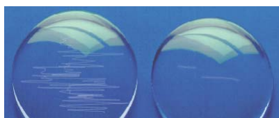
Abrasion testing shows an increase of 2 to 3 times in Bayer Ratio results over traditional AR. Bayer results vary from 4 to 9 depending on the underlying lens brand.
